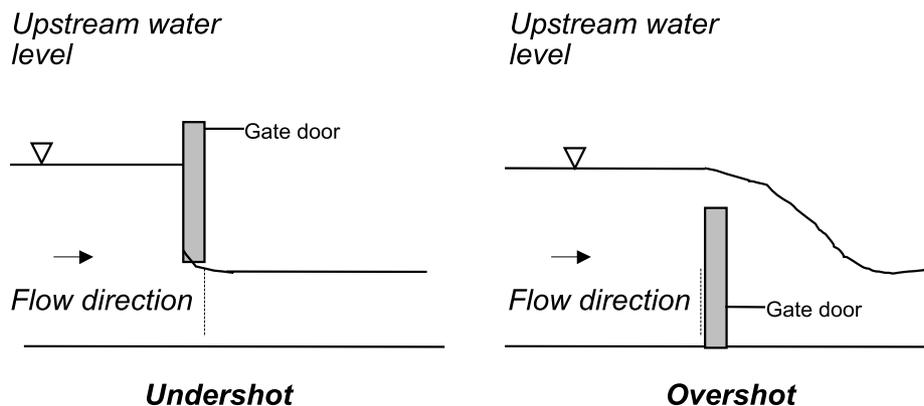
**Figure 1.** Illustration of under and overshot operation of the main regulator.
